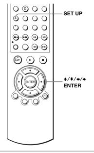
Press SET UP, then press **♦/♦** to select (OPTION) and press ENTER.
